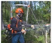
Flexible saw suspension The saw has a flexible suspension for less fatigue and increased comfort.
